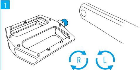
One of the pedals has a right- and the other a left-hand thread. Most pedals have the letter "L" and "R" stamped on the end of the thread. Some pedals come with a groove in the flange of the left pedal.
