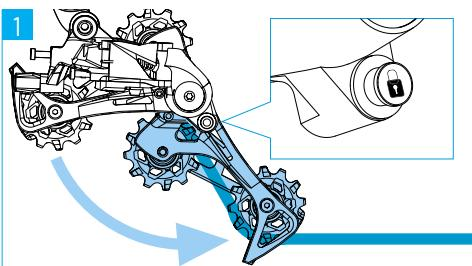
Activate the Cage Lock function. Pull the cage of the rear derailleur forward and press the Cage Lock button with the symbol
