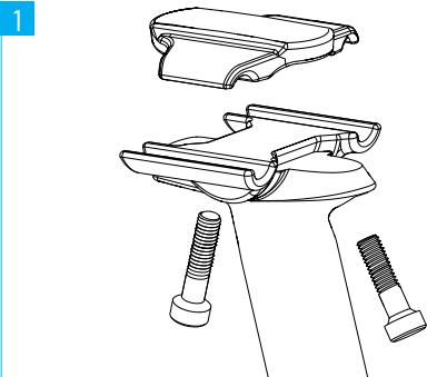
Unscrew the bolts of the saddle clamp and remove the upper clamp.
