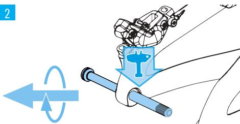
1. Remove the thru axle from the frame.
