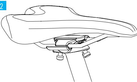
1. Attach the upper clamp to the saddle frame.
