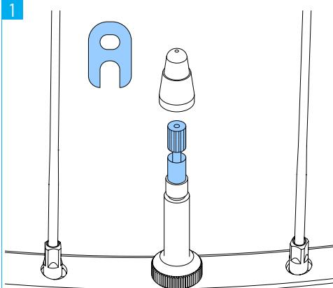
1. Release the air from the tire completely.
