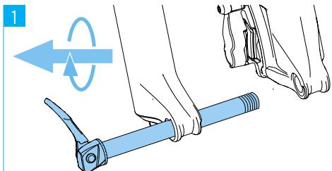
Remove the thru axle from the fork.
