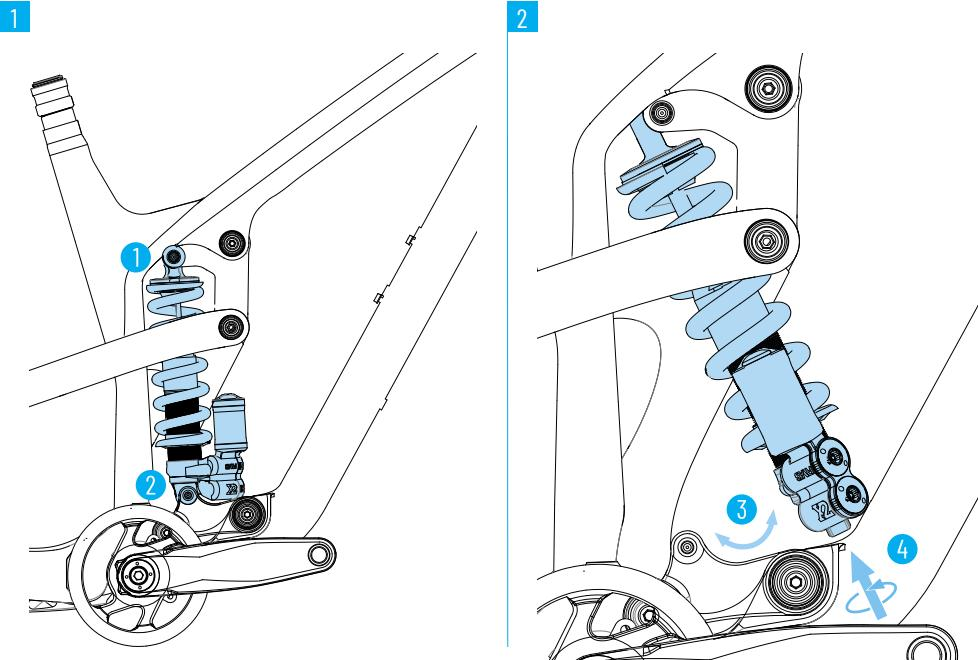
1. Loosen and remove the upper shock bolt first. Pulling out the bolt is made easier by slightly lifting the rear end.
