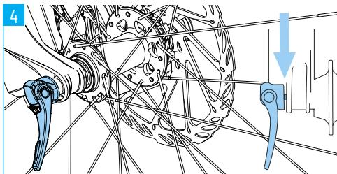
Rotate the lever clockwise until there is only a small gap left between lever head and dropout.
