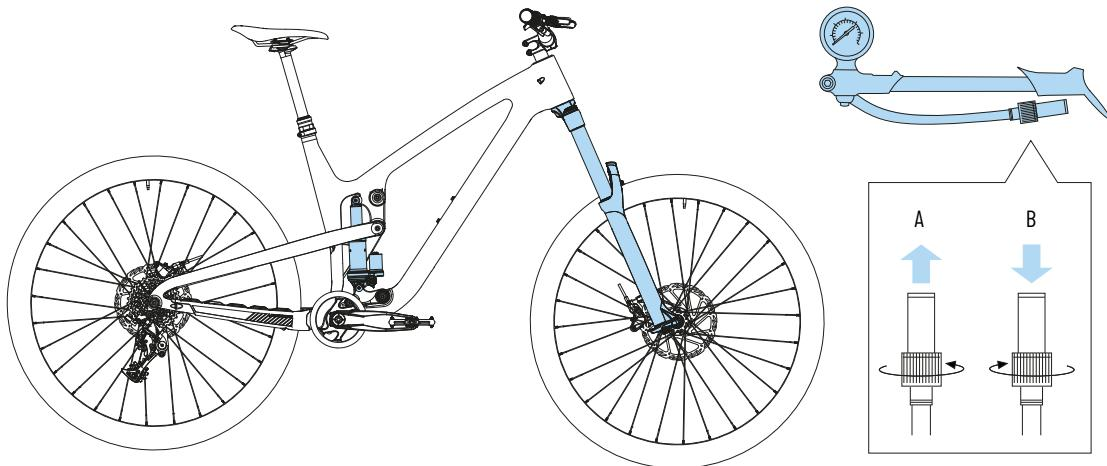
1. Unscrew the valve cap of the shock / fork.
