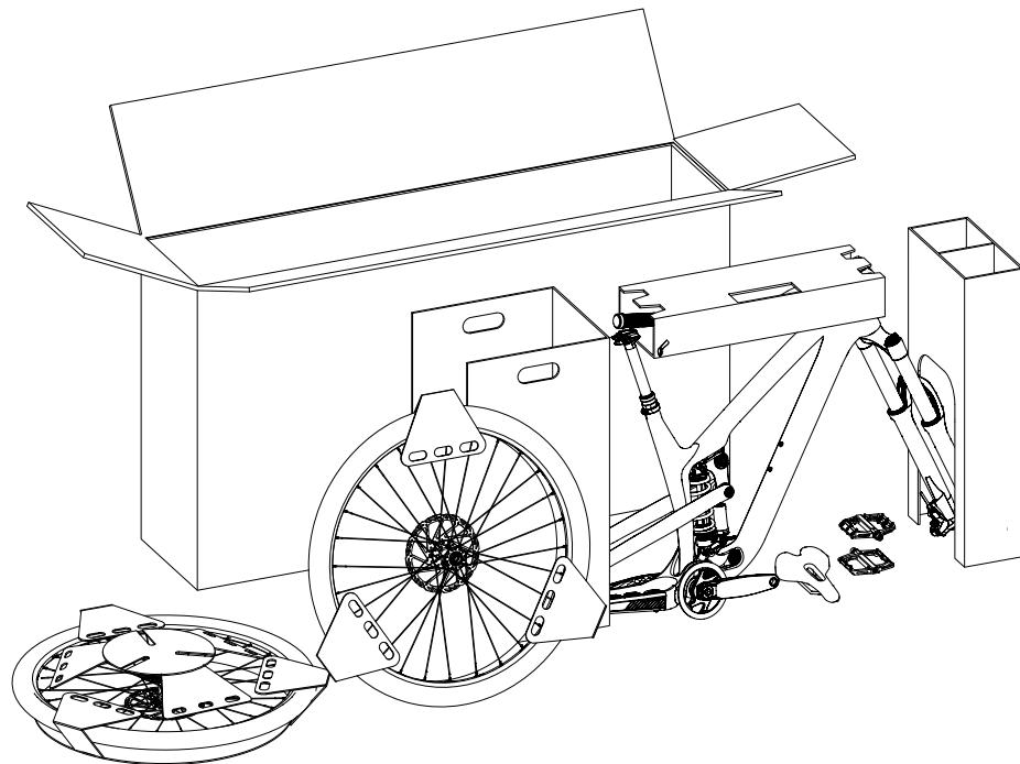
1. Secure or cover all loose or moving parts properly. Sharp or pointed components have to be wrapped additionally to make sure they won't damage other parts of your bike and won't tear through the outer packaging.
