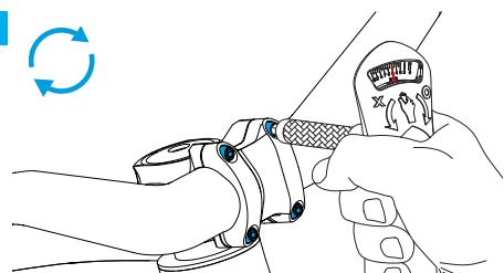
1. Screw in the two upper clamping bolts and tighten both bolts with the torque lasered on the clamp or stem.
