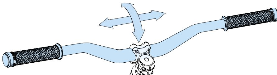
1. Center the handlebar and adjust the angle of the handlebar according to your personal preferences.
