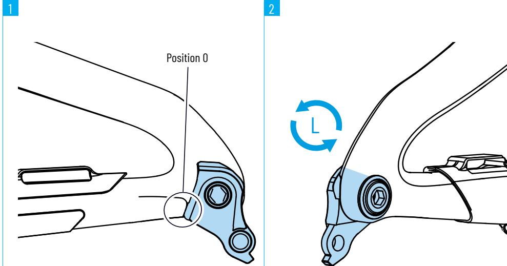
1. Insert the UDH derailleuer hanger from the inside into the dropout of the frame.
