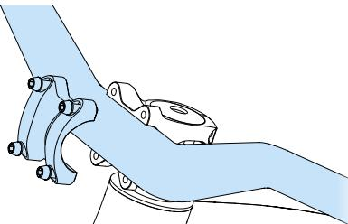
1. Attach the handlebar to the stem.
