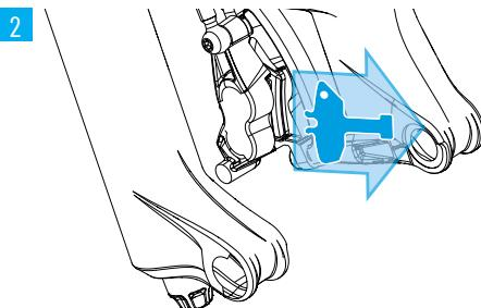
1. Remove the transport securing device that is fitted between the brake pads.
