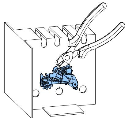
Detach the rear derailleur from the rear end fixation.
